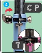
With the QR in the open position, tighten the nut manually until a position where the QR lever leaves you a slight pressure mark in the palm of your hand after closing it.
