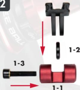
Install lamp base and 1-2 to fit 1-1, and use 1-3 to screw together.
