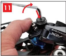
**11** Use the 4 mm hex wrench to tight both pieces together (8 N.m). Hold down the Cam Unit and the Stabilizer Unit during the process so they do not move.
