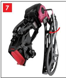
Use the 3mm hex wrench to fix the body to the OSPW evo. Tight to 4 N.m.
