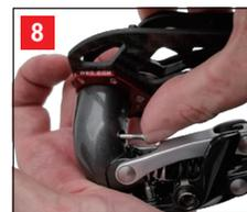
Keep holding both pieces together and reinstall the body screw. Tight (2 N.m) it with a 2 mm Phillips screwdriver.
