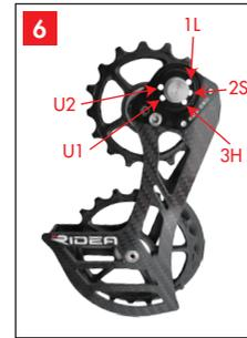
2S is the Standard tension setting and the one we recommend to start with. Then, in case you need lower tension and friction on the chain you can switch to 1L, which is the Low tension setting, to see if that works better for you. On the contrary, in case you want better shifting performance, you can switch to 3H, which is the High tension setting, to see if the increased tension and friction of the chain works for you.
