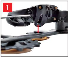
Turn clockwise the high limit screw to separate the body from the pulley cage.
