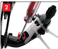
Use a 2 mm Phillips screwdriver to release the partly threaded body screw.
