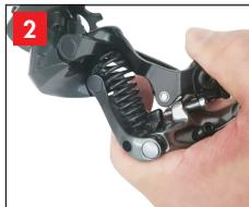
First of all, please expand the four bar linkage of rear derailleur cage to maximum position.
