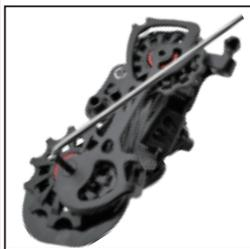
2 Disassemble the original rear derailleur cage and pulleys.
