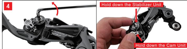
Use the 4 mm hex wrench to remove the pulley cage. Hold down the Cam Unit and the Stabilizer Unit so they do not move. After removing the pulley cage, press down the Cam Unit and the Stabilizer Unit to make sure they are in position.
