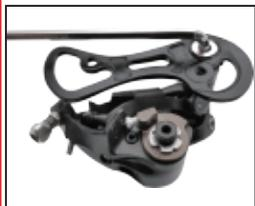
**3** Disassemble the original cage.
