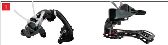
To facilitate access to the body screw, extend the derailleur body and fix it in extended position with cable ties. If you are working with the derailleur installed on your bike, just shift to the largest cog.
