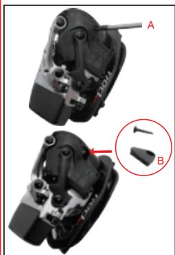
2 Use T7 star key wrench to remove rear triangular plate of rear derailleur cage.
