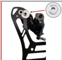
**12** The side cap's gap of upper pulley must be aimed at fixing bolt.
