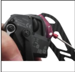
**11** Use a 2.5 mm hex wrench to assembly the pulley cage stop screw (tight to 1 N.m). Then use the same tool to assembly the pulleys (logos facing outward) and the inner cage (tight to 2.5 N.m).
