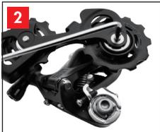
Use 2.5mm hex wrench disassemble the original rear derailleur cage and pulleys.
