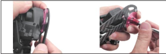
**10** Press down gently and at the same time turn the outer plate clockwise slowly. Keep doing this until you align both "D" shapes so they can fit into each other. This should be when the pulley cage stop screw position reaches the stopping position in the rear derailleur. Hold down this position and use the supplied special extractor tool and a 5 mm hex wrench to tight the outer plate. Tight to 2.5 N.m.
