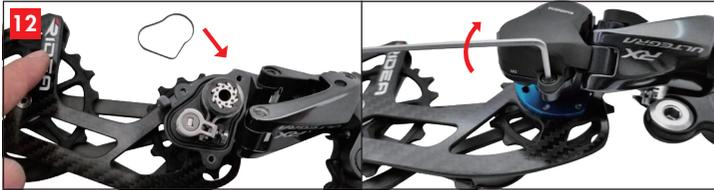
Reinstall the rubber ring to its original position. Reinstall the P-Cover back to its place (press down to their original position the Cam Unit and the Stabilizer Unit in case they impede placing the P-Cover back) and use the 3 bolts to secure it (1-1.5 N.m)
