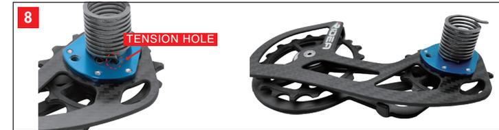
Insert the hook of the P-Tension spring on the tension hole of the OSPW evo.
