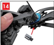
**14** Reinstall the pulley cage stop screw (1 N.m).
