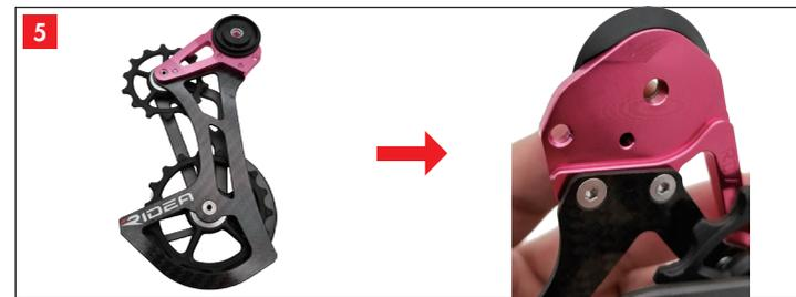
Put the spring base on the adaptor. Fix the base on the position as illustrated.
