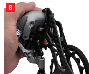
Turn to fixed position and hold the derailleur and plate.
