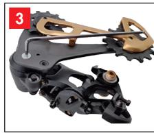
Use the 3mm hex wrench to remove the body screw and get access to the spring compartment.
