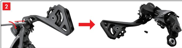
Remove the plate stopper pin with a screwdriver. Carefully allow the pulley cage to unwind. This will release the tension from the spring. Your derailleur should appear as in the photo.
