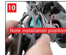
Align the extreme of the spring with the groove in the body cage and insert it with the OSPW evo. Hold both pieces together.
