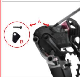
**10** Assemble rear triangle plate, use T7 Star key wrench to tighten the screw on triangle plate lightly. (Please do not overtighten, or the screw may get stripped.)
