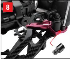
Reinstall the pulley cage stop screw (tight to 1 N.m).
