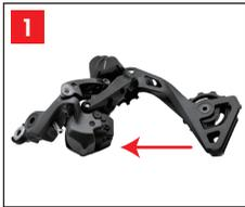
Make sure that the lever switch is in the OFF position. If necessary, move the derailleur body outwards so it leaves free way to the pulley cage.
