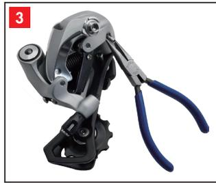
Use the needle nose pliers to take out the tenon after rotating.
