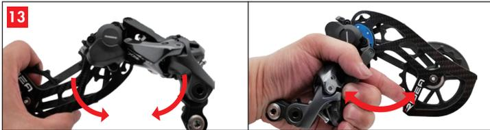
Turn the derailleur body clockwise and the OSPW evo counterclockwise to return the derailleur to its resting position. Please note turning directions to avoid any damage.
