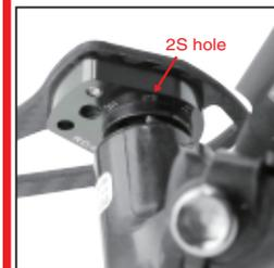
**9** Fix the front cage plate after choosing the corresponding spring tension.
