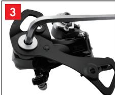
Use 5mm hex wrench disassemble the original cage.
