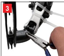
If required, use a needle nose plier to remove the body screw. **(Attention: Before you fully remove the body screw, please press the pulley cage against the derailleur to avoid an abrupt release of the spring tension.)** Carefully allow the pulley cage to unwind, opening the spring compartment.
