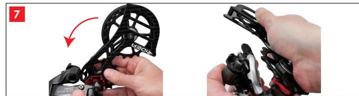
Gently hold both parts together and rotate counterclockwise the OSPW evo until the pulley cage stop screw overpass the bulge of the derailleur body. Then press firmly to fully insert the OSPW evo into the derailleur body.
