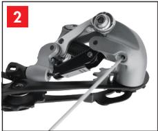
Use 2mm Hex wrench to take out the tenon of Shimano 105 rear derailleur cage.
