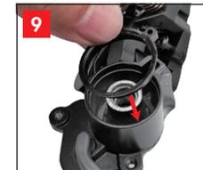
Place the P-Seal ring into the derailleur body.
