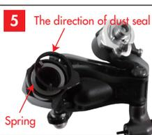
Dust seal has directional sides, fix the narrow side of seal downward into rear derailleur's body.
