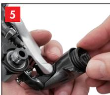
Insert the tension spring in the derailleur body and make sure that the internal hook is inside the tension hole.
