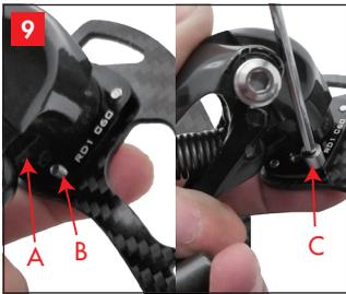
Fix the limit screw. Please fix the limit screw in front of the stopper.
