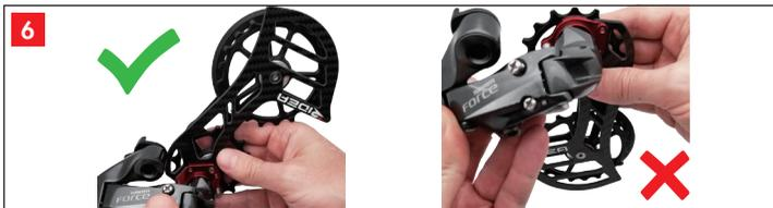
Align the external hook of the spring with the correct group of tension holes of your OSPW evo (see note below). To know which group of tension holes is the correct one, when aligning your OSPW evo with the spring, it should form an angle of approx. 90° with the derailleur body and the lower pulley should be pointing up and forward. Choose the proper hole according to your tension preferences (see note below) and insert the spring hook in it.
