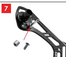
Take limit screw out and divide to M3 bolt and nut.
