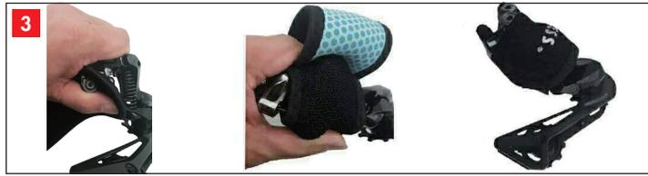
As shown in the illustration: For disassembling easily and make more space between the cage and the body of rear derailleur. Please use velcro tie or nylon cable tie etc. to fix the four bar linkage and keep the position.
