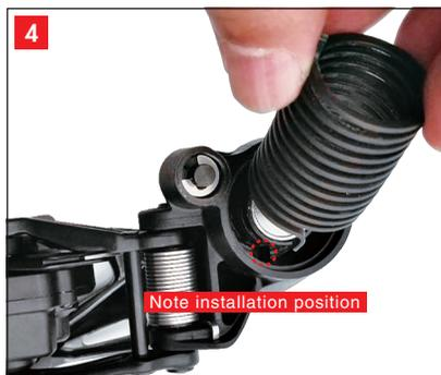
Be sure that the tip of the spring remains in the installation hole of the body. Place it properly if it moved when you removed the pulley cage.
