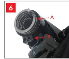
Warning: Please fix the spring first, and then fix the dust seal.
