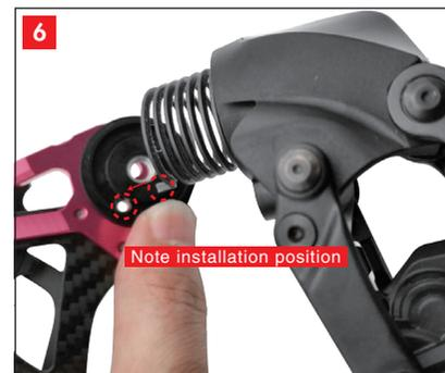
Place the other tip of the spring in the tension hole of the OSPW evo and compress the spring to close the gap.
