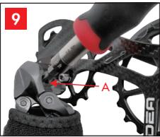
Fix the T10 Torx screw tightly.
