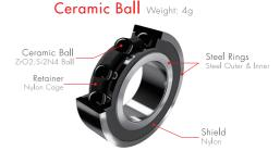
The combination of steel rings and ceramic balls offers better durability and rotation capabilities than full steel bearings, with a slightly more demanding maintenance and weight penalty when compared full ceramic bearings.
